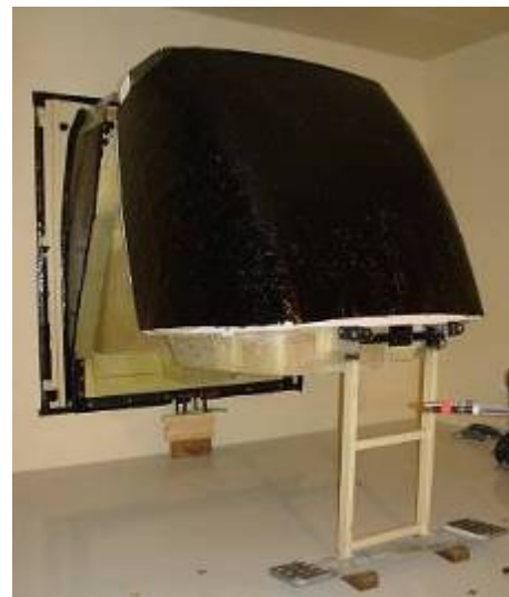
Figure 4. Tram cabin fitted between the two rooms. The areas not studied are masked with heavy load.
