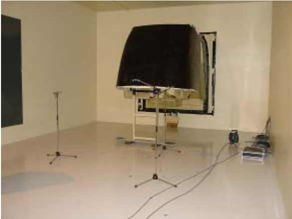
Figure 1. Emission room with tram cabin.
