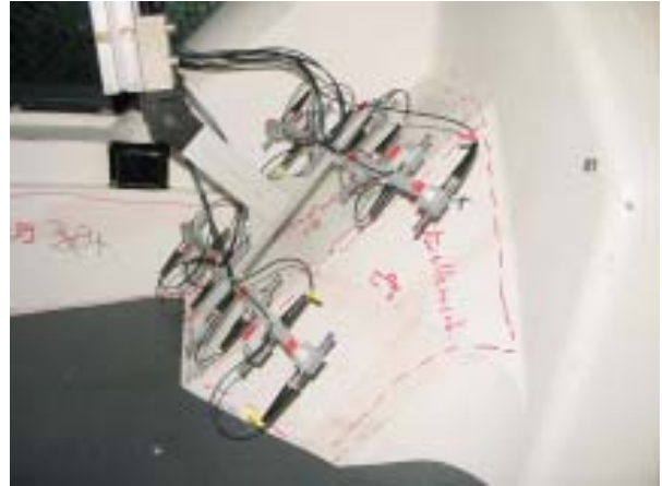
Figure 3. Microphone measurement antenna on support.
