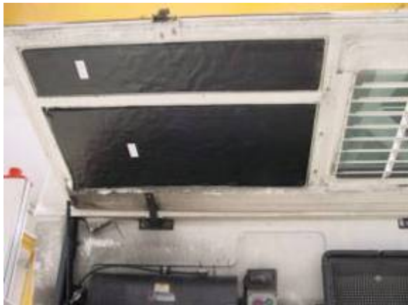
Figure 5. SILENT CUSHION fitted on backside panel.
