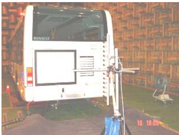
Figure 1. Acoustic antenna measurement in semi-anechoic-room.
